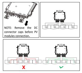
Step 8. Connect APsystems Microinverters to Grid
