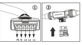
Step 6. Install a Bus Cable End Cap at the end of AC bus cable
